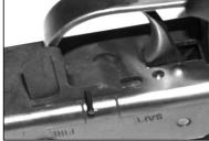
3) To protect the finish, place a piece of tape on the trigger guard side of the extended safety. Place extended safety on lower receiver, over safety stub.
