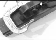
4) Using a 1" C-clamp, place the fixed part of the clamp on the roll pin and position the swivel side on the other, over the tape. Tighten the C-clamp and drive the roll pin into the extended safety until it is flush. Remove C-clamp and tape. Re-assemble M-11/9.
